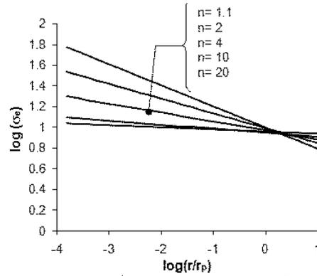
Figure 3: Radial variation of the asymptotic normalised plane-strain equivalent stress for the interfacial free-edge ( $\theta_0 = 60^\circ$ ) at  $\theta = 30^\circ$  for different hardening exponents
