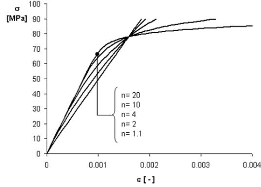
Figure 2: Non-linear Ramberg - Osgood material behavior
