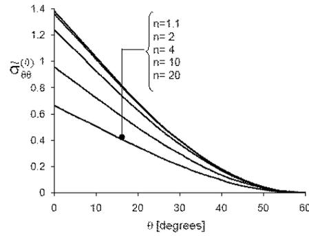
Figure 6: Angular variation of the asymptotic normalised plane-strain radial stress component  $\tilde{\sigma}_{\theta\theta}^{(0)}$  for the interfacial free-edge joint ( $\theta_0 = 60^\circ$ )
