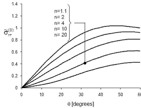
Figure 5: Angular variation of the asymptotic normalised plane-strain radial stress component  $\tilde{\sigma}_{rr}^{(0)}$  for the interfacial free-edge joint ( $\theta_0 = 60^\circ$ )
