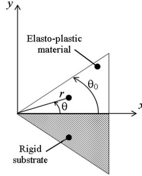
Figure 1: Geometry of interfacial free-edge joint and cylindrical coordinates
