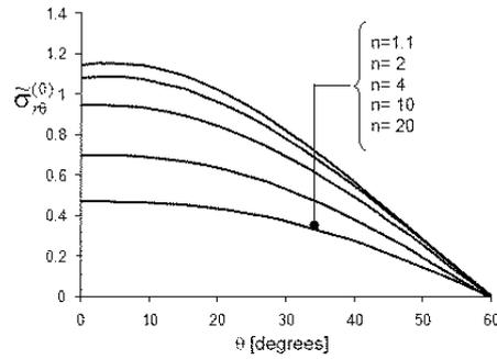
Figure 7: Angular variation of the asymptotic normalised plane-strain radial stress component  $\tilde{\sigma}_{r\theta}^{(0)}$  for the interfacial free-edge joint ( $\theta_0 = 60^\circ$ )
