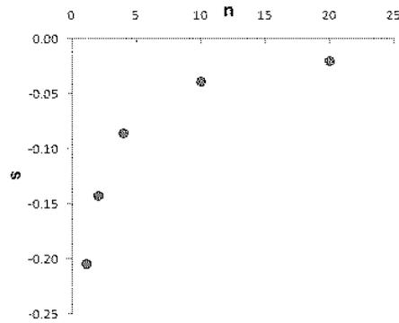
Figure 4: Singularity order versus hardening exponents for the interfacial free-edge ( $\theta_0 = 60^\circ$ )
